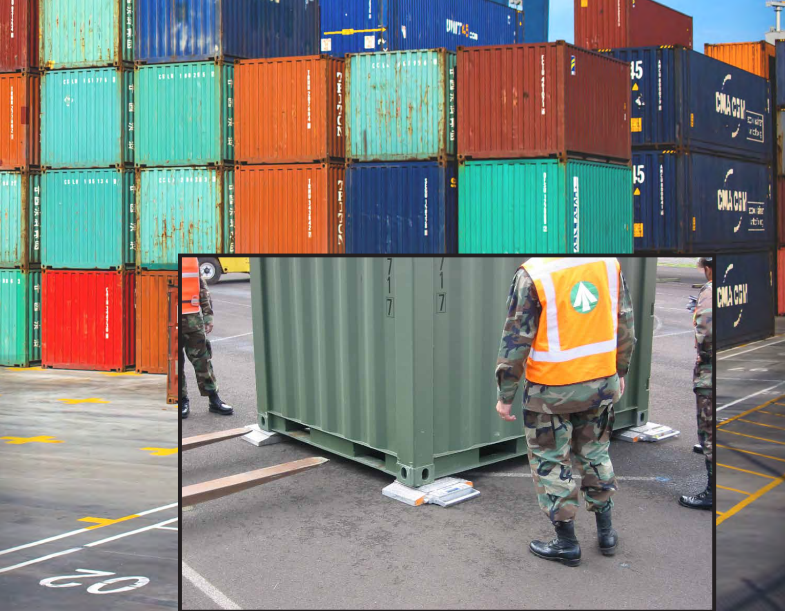
A shipping crate is positioned onto four Intercomp aluminum RFX™ Wireless PT300™ electronic scales while port authorities prepare to log in the weight in accordance to the SOLAS method1. These fully equipped scales are capable of weighing up to 20,000 lbs and come standard with solar charging panels.
