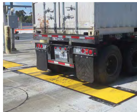
Top: In ports that need weigh-in-motion applications, Intercomp's minimally invasive installation WIM strip sensors are available for both low and higher speeds. Below: For low speed weigh-in-motion applications the LS-WIM Axle weighing scale from Intercomp is the best choice. Both are SOLAS Method 1 options.
